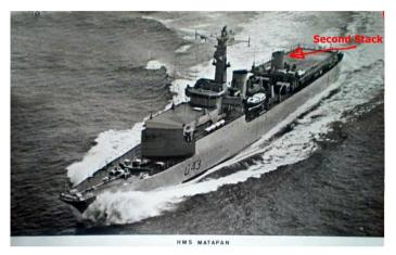
Whilst on sleek conversions, one that twanged my thong was the ex. Battle Class Matapan. She became the Admiralty 'sonar trials ship'. A second funnel fitted is not distinct in my small pic. when enlarged. It was the exhaust for installed extra generation capacity. I can imagine the draughtsman in Pompey dockyard when given the task, he must have been an old romantic to put that lovely 'clipper bow' on her.
